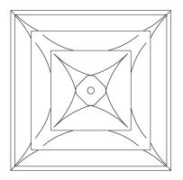
**Duct Diameter (in.):** 14 Backpan Height (B): 2.5" Cone Depth (C): 1.063" Nom Ceiling Module: 24"x24"
