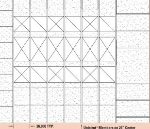
(as shown) and hospital rooms present unique challenges to ceiling design due to the specialized equipment required. This equipment is typically hung from a metal framing support system (example Unistrut®) mounted in the ceiling and requires close coordination to ensure fitment. Contact Price for design assistance.
